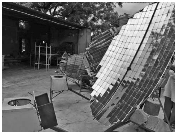
Photograph 4 The parabolic Scheffler solar cooker fabricated by women at Barefoot
